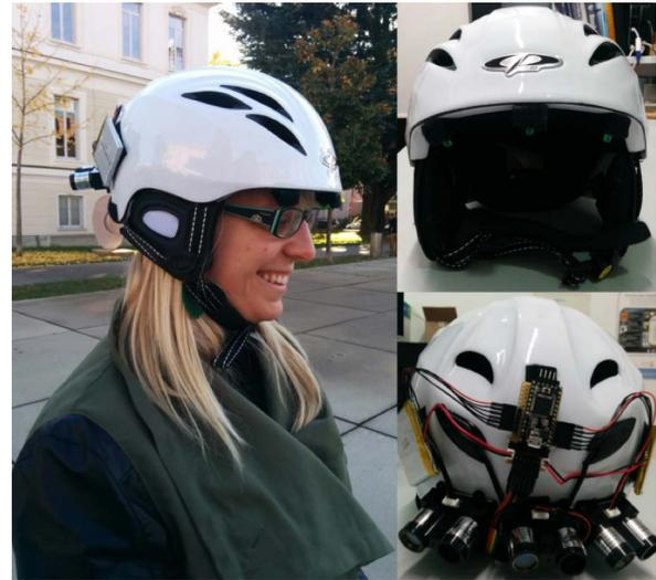
Figure 1. Left: A user wearing S-SH. Top right: Front view of S-SH with 3 LEDs feedback system. Bottom right: Back view of S-SH with 3 LIDAR sensors, a control unit and 2 batteries.
