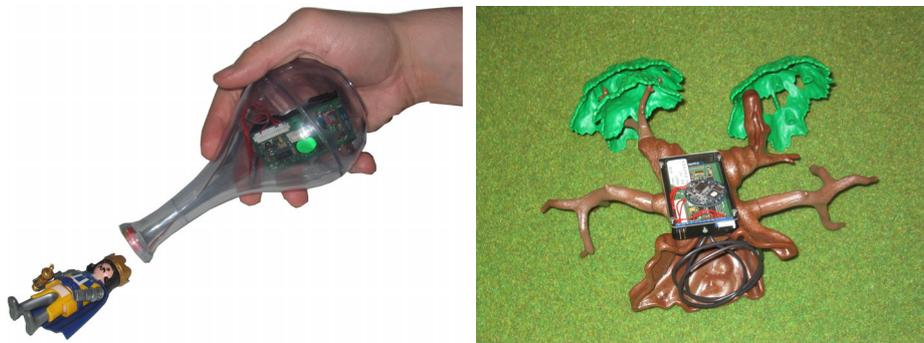
**Fig. 2.** The „magic potion bottle”, a smart toy equipped with a BTnode, acceleration sensors and a mobile RFID reader; the magic potion can be administered to a figure (the RFID tag is integrated in its head) after having been shaken „well enough” (left). The „magic tree”, a movable landscape element equipped with a BTnode and a mobile RFID reader (right).
