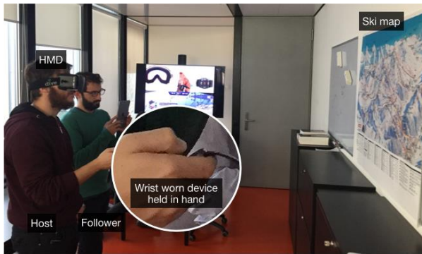
Figure 5: The laboratory setup of the SkiAR system
