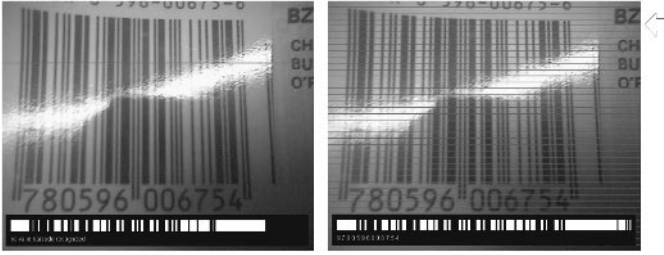
Figure 1: Multiple scanlines : In contrast to existing approaches, we make intense use of multiple scanlines in our algorithm to both increase robustness and improve accuracy. While the image shows all of the scanlines oriented in parallel, our system supports any orientation of scanlines.
