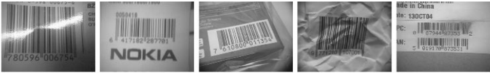
Figure 3: Successfully recognized codes : The above pictures show that our algorithm can handle reflections and shadows as well as slightly crumpled paper.
