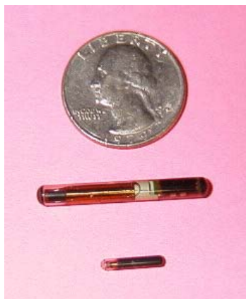
Figure 3: Typical form factors for RFID tags. The particular tags shown come in a glass casing in order to allow attaching them to metallic objects or to insert them below the skin of animals. (Image Source: Portolano Project [13])
