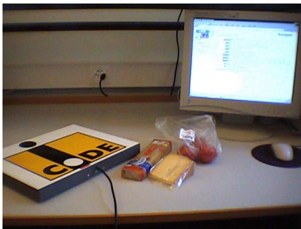
Figure 5: Experimental setup of RFID Chef in our lab. A standard office desk functions as our kitchen counter, an 18” LCD monitor acts as our display. Several individual ingredients have been placed on the table, where an RFID antenna (here shown in its casing, next to the ingredients) detects them and reports their presence to a PC that controls the display. Note that the antenna is usually mounted underneath the table.
