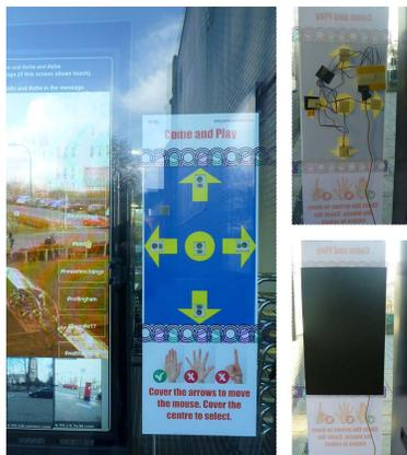
Figure 7: An actual example of installed Light-Keypad. Left is front view; up-right is internal back view and bottom-right is the back view with a cover
